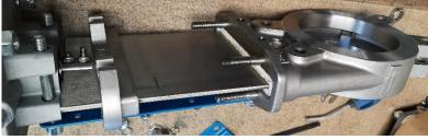
Packing are linear type joined together. With a plane screwdriver, get the packing out of the body. There
