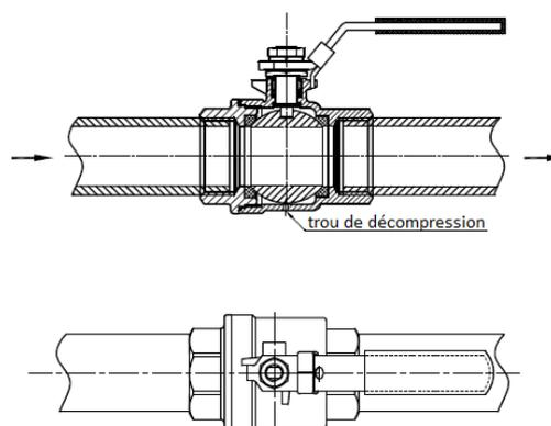
**ROBINET A TOURNANT SPHERIQUE INOX 2 PIECES A DECOMPRESSION BSP**
